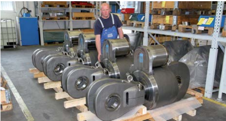
Final inspection of snubbers type 31
