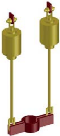
LISEGA standard supports in SmartPlant® 3D
